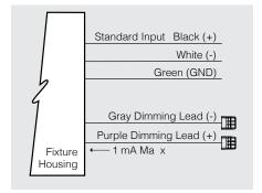
Driver has a 0-10V dimming interface with dimming range of 10-100%. Is compatible with most control systems including Hubbell Building Automation wiSCAPE™, Controls compatible via Gray and Purple dimming lead.
