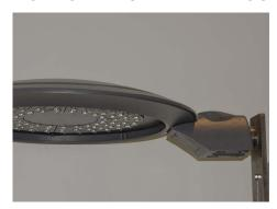
Optional horizontal slip-fitter arm is available for mounting to a 1-1/4" to 2" pipe-size mounting end (1-5/8" to 2-3/8" OD). The casting has a ±5° adjustment to accommodate davit arms that are not horizontal.
