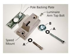
Speed mount assembly. Standard washers (A) and shoulder washer (B) must be used when threading mounting bolts into pole backing plate to assure that luminaire is mounted securely to pole.
