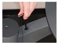
**1.** With 5mm hex wrench, partially loosen embedded top bolt.
