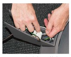
**10.** Connect wires (voltage to black, white to common, green to ground) directly into the terminal block.
