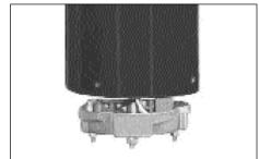
6. Place the pole body over the base casting and slowly turn until it drops into retaining slots. Then, twist clockwise 45 degrees to lock pole onto base casting.
