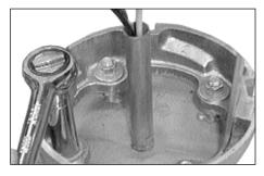
3. Tighten the upper nuts using a 9/16" deep socket
