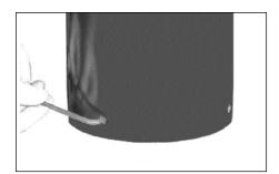
7. Tighten two 3/8" set screws at the bottom of the pole using a 3/16" hex key.
