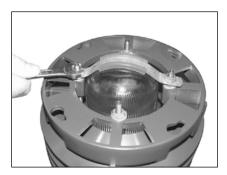
**12.** Using 7/16" wrench, attach louver cap and retaining strap to louver stack using 1/4-20 nuts.
