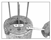
Pull quick-disconnect from driver assembly through hole in center of mounting plate. Use 7/16" wrench, secure mounting plate to riser with four 1/4-20 hex bolts provided.
