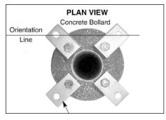
not be in contact with soil or other corrosive elements. If luminaire will not be installed on lit bollard, cover top of bollard so water and debris will not collect inside.
