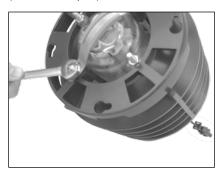
**6.** Using 7/16" wrench, remove two 1/4-20 nuts securing retaining cap.
