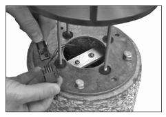
10. Join the disconnecct plugs between the optical assembly and driver assembly. Tuck disconnect plugs and extra wire inside riser, taking care to avoid wire pinching.
