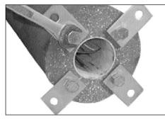
Install four anchor plates using 15/16" wrench with four 5/8-11 hex head bolts povided. Position the anchor plates straight from center on round bollards (see plan view below).
