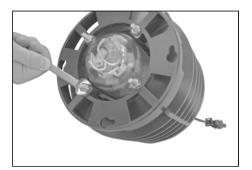
Continue to remove four 1/4-20 nuts securing louver stsck. Remove louver stack and set aside.
