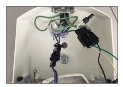
Connect incoming wires from housing to corresponding connectors on new driver assembly.
