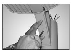
**3.** Install arm access cover and secure with self retained screw using a B " Allen wrench. Be sure wires are not pinched as screw is tightened.
