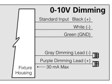
Driver has a 0-10V dimming interface with a dimming range of 10-100%. Is compatible with most control systems including Hubbell Building Automation wiHUBB<sup>™</sup>. Approved dimmers include Lutron Diva AVTV, Lutron Nova NFTV and NTFTV. Note: Not compatible with current sourcing dimmers. Controls compatible via Gray and Purple dimming lead.
