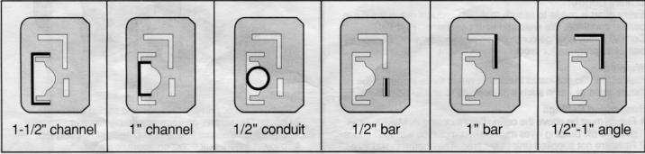
Rail supports accept many types of rails. Job site scrap can be used to support fixtures.
