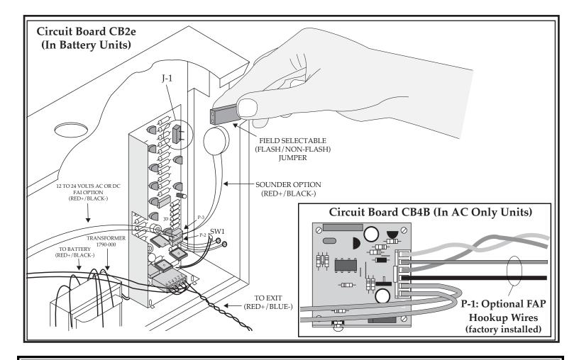
ALL BATTERY UNITS HAVE (FIELD SELECTABLE) EMERGENCY FLASHING OPTION If you want the unit to flash during AC power failure, place jumper (see above) on only the upper post of J-1. If you want the unit to stay on solid during AC power failure, place jumper across both posts of J-1.
