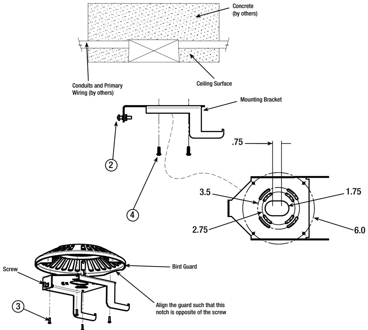
5. Hook the Orbeon housing on to the bracket.
