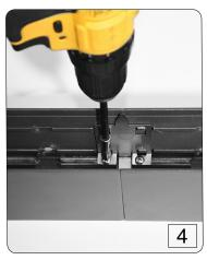
Align the next housing unit into the other half of the mating plate and repeating step 3.
