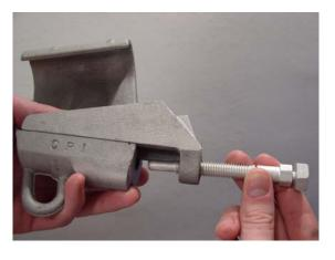
3) Make sure threads are clean and install a new shear bolt.
