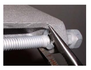
5) Squeeze snap ring into the slot until it is securely fastened.
