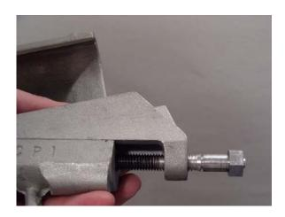
2) Fully remove existing shear bolt.
