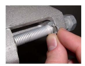
4) Align the new snap ring into the existing slot on the shear bolt.
