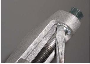
1) Insert screwdriver blade under the snap ring and use a twisting motion to pry it out.
