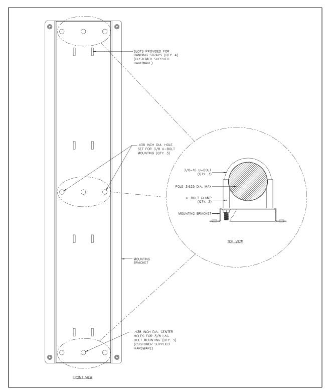
Figure 1. Pole Mounting Bracket Installation Detail
