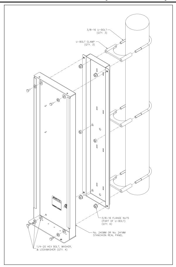
Figure 2. Bracket and Enclosure Installation
