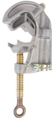
C6001733 Aluminum body, Smooth jaws, Bronze eyescrew with Acme threads, Tapped for 3/8"-11 UNC threaded ferrule
