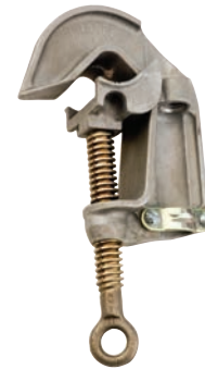
T6003203 Aluminum body, Smooth jaws, Bronze eyescrew with Acme threads, Tapped for 5/8-11 UNC threaded ferrule
