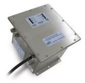
The Austdac UPS (Uninterruptible Power Supply) uses Ni-MH (Nickel metal hydride) batteries. The Austdac UPS design minimises the stress on the Ni-MH batteries by ensuring the batteries are charged at a lower rate and not fully discharged while monitoring each cell and overall temperatures. Ni-MH batteries do have a limited life as stated by battery manufacturers such as Energizer who state in their Nickel Metal Hydride (NiMH) Handbook and Application Manual that ;
