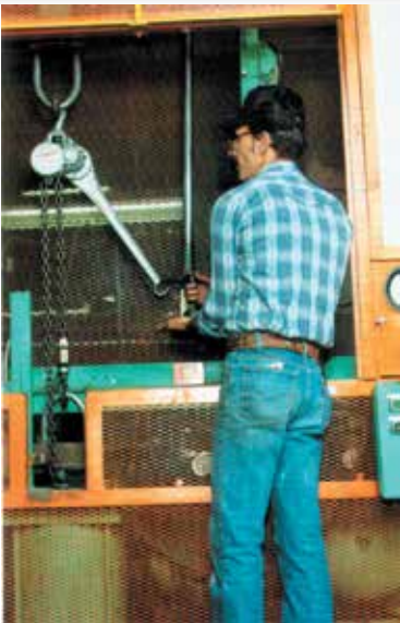
Chance® hoists are pull-tested before leaving the factory.
