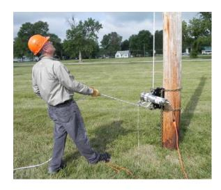
The Chance® hoist is equipped with an anti-reversing brake which keeps the drum from turning backwards. This allows the load to be held in position by holding the fall line. If the load needs to be lowered, simply allow the rope to slip back around the drum slowly, allowing the operator to lower the load safely and in full control.
