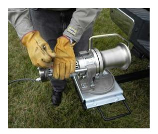
Always mount the hoist to the proper bracket using the high strength bolts and fasteners supplied with each hoist. If fasteners are damaged or missing, replace them with the same type and grade designation. The fasteners must be tightened evenly to the proper torque to insure "load sharing" by all the fasteners.
