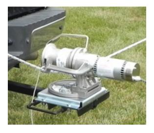
The rope to be used over a capstan drum needs three things: adequate working load, good frictional characteristics, and high temperature melting point. As rope goes around a capstan drum, it must slip a small amount to advance across the drum. This creates friction which causes the drum to heat. If the drum is allowed to rotate without advancing the rope, heat builds up quickly and melts plastic ropes.
