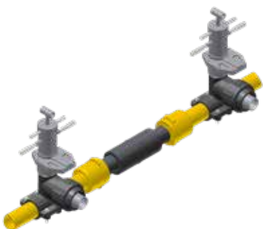
10. Move sealing element to outlet. Remove PE pipe by-pass
