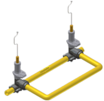
3. Remove abandonment nuts and replace with compression nuts
