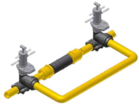
9. Repair damaged pipe
