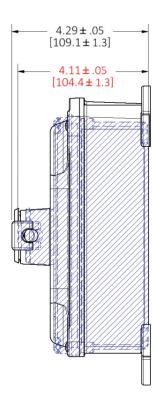
30A enclosure shown above. Legacy HBLDS3 measurements in red. Light blue shading is legacy enclosure. Mounting patterns are the same.
