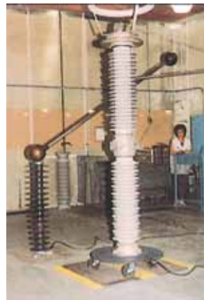
Routine quality control testing of station class arresters.
