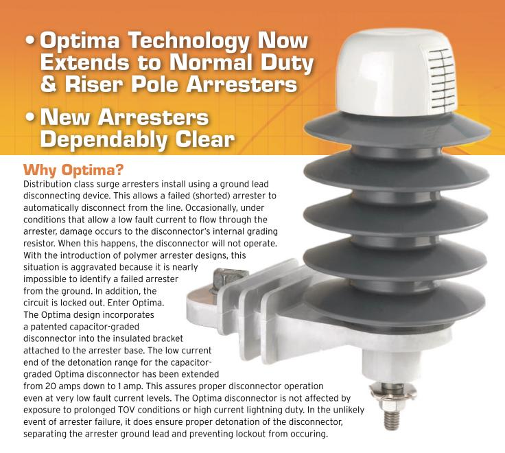
Don't let shorted arresters get in the way of your reliability. The Ohio Brass (OB) Optima arrester resolves service interruptions caused by shorted arresters immediately and gives crews a "heads-up" by showing the line lead that's disconnected at the lower terminal of the arrester.
