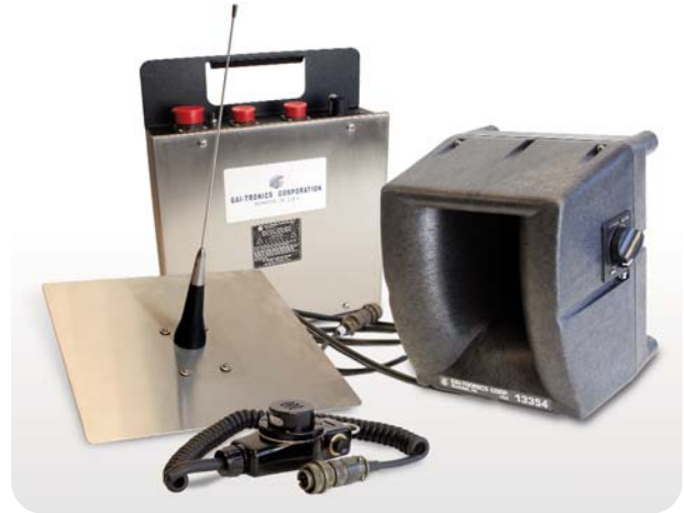
Components of GAI-TRONICS Industrial Radio System include: Transceiver with power cord; ground plane antenna; handheld dynamic microphone; and wall mountable loudspeaker with volume control.
