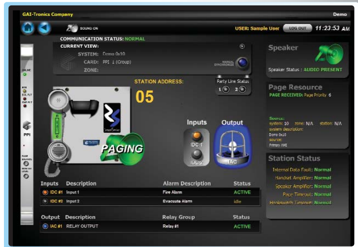
SmartSeries RTU Station View: Healthy with paging and active input/output
