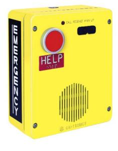
Although each of these telephones will function as a standard Emergency Telephone, connecting a customer-provided, central computer equipped with GAI-TRONICS' TMA (Telephone Management Application) software will allow them to operate in SMART (**S**elf-**M**onitoring **a**nd **R**eporting **T**echnology) mode. With TMA connected, each RED ALERT® telephone will be polled on a scheduled basis to report:
