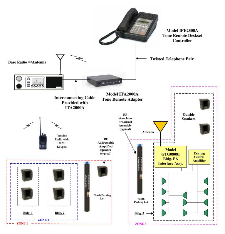
Notes: 1. Each Addressable Amplified Speaker will require 120 Vac (12 Vdc power supply) or solar power.
