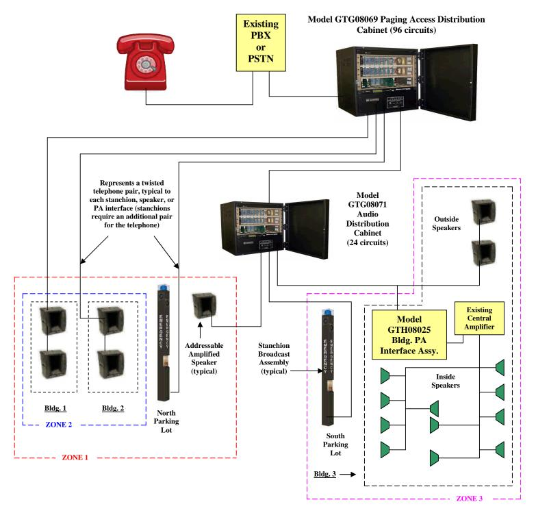
Notes: 1. Each Addressable Amplified Speaker will require 120 Vac (12 Vdc power supply) or solar power.
