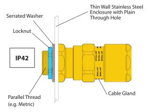
Thin walled stainless steel enclosure with a plain clearance hole, no additional sealing and secured with a locknut and serrated washer – This will be expected to maintain IP42.
