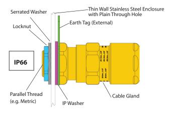
So long as the earth tag is flat, does not bow away from the compression face of the entry and the mounting holes are perpendicular then this arrangement may be expected to meet IP66.
