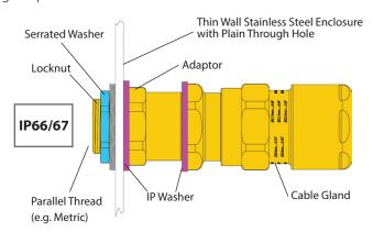
By adding a sealing washer between the adaptor and gland entry, the arrangement will be expected to meet IP66 and IP67.
