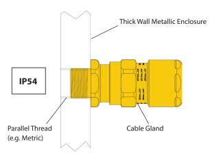
Parallel threaded metric joint with no additional sealing – This may be expected to maintain IP54 in line with EN 60079-14 Clause 10.6.2 (min 6mm wall thickness)
