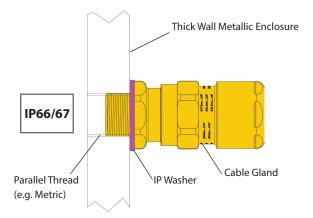
Parallel threaded metric joint with Hawke IP washer – This may be expected to maintain IP66 and IP67. Note the conditions of the enclosure mentioned earlier in this document.
