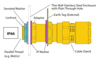
If an earth tag is fitted between the nylon washer and the cable gland, so long as the earth tag is flat and does not bow away from the compression face of the entry then this arrangement may be expected to meet IP66.
