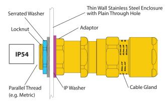
As there is no additional sealing between the adaptor and the gland entry, the threaded joint can be expected to maintain IP54.
