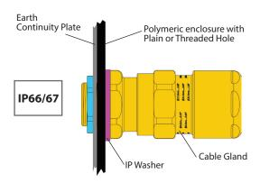
Thinwalled polymeric enclosure with a plain clearance hole, fitted with a nylon sealing washer and secured with a locknut – This will be expected to maintain IP66 and IP67. Be aware of limitations regarding maximum hole size. These normally form part of the special conditions of use of the enclosure.
