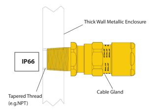
A 'wrench tight' Tapered NPT threaded joint may be expected to achieve IP66. If being used in an application where ingress is a concern, additional thread sealant may be used so long as it is allowed by the protection concepts of the installation.
