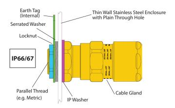
If the earth tag is fitted internally to the enclosure, it will not have any impact on IP, therefore this arrangement may be expected to achieve IP66 and IP67.
