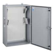
R Industrial REBOX<sup>®</sup> is a NEMA type 4, 12 and 13 enclosure that is designed for harsh environments to protect housed contents from oil, dirt, dust, moisture and outdoor elements. A specially designed mounting plate at the rear of the enclosure allows mounting of standard REBOX<sup>®</sup> accessories, brackets and kits.
