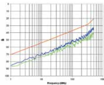
**PSNEXT:** The unwanted signal coupling from multiple transmitters at the near-end into a pair measured at the near-end.
