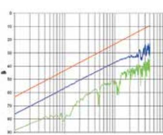
**ELFEXT:** A measure of the unwanted signal coupling from a transmitter at the near-end into another pair measured at the far-end and relative to the received signal level.
