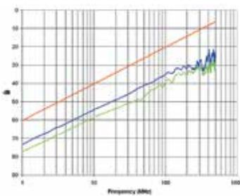
**PSELFEXT:** A computation of the unwanted signal coupling from multiple transmitters at the near-end into a pair measured at the far-end and normalized to the received signal level.
