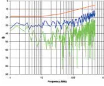
**Return Loss:** Ratio of the signal reflected back at the transmitter relative to the original signal sent. In a full duplex application, like 1000BASE-T, significant Return Loss can cause network errors.
