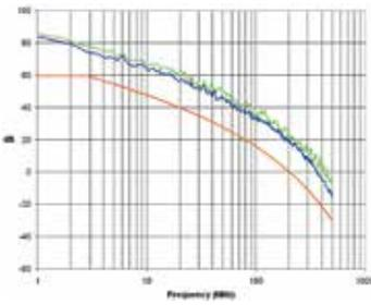
**PSACR:** Difference between the attenuation and the Power-Sum NEXT at a given frequency (signal to noise ratio). Available bandwidth is the point where PSACR is equal to zero.
