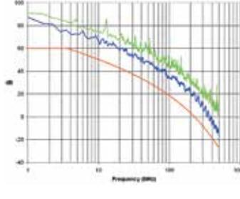
**ACR:** Difference expressed in dB between the signal attenuation produced by a cable and the near-end crosstalk (NEXT).
