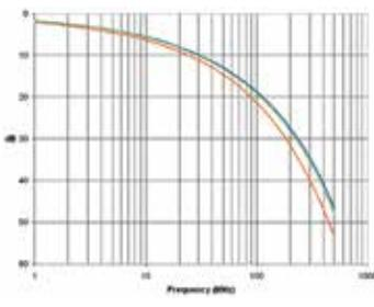
**Attenuation:** The decrease in magnitude of transmission signal strength between points, expressed in dB as the ratio of output to input signal level.
