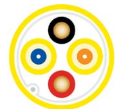
Hybrid cable cross-section
