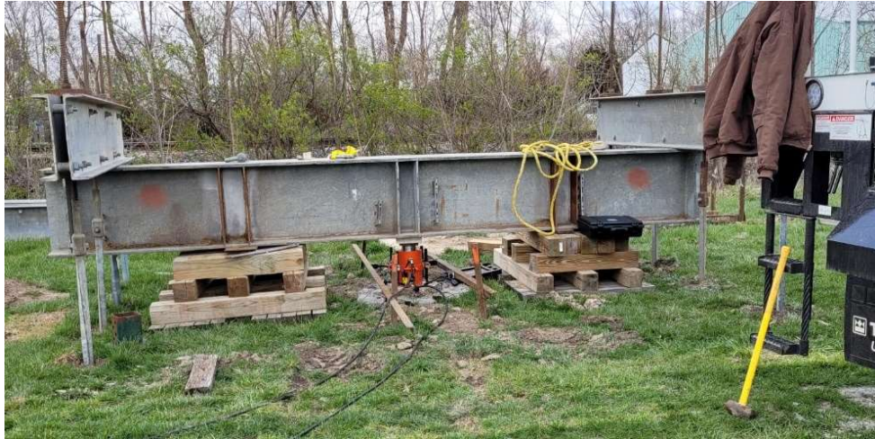
Photo 3: Typical Compression Test Setup
