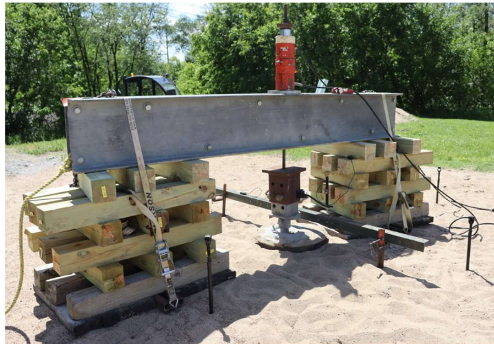
Photo 4: Tension Test Setup
