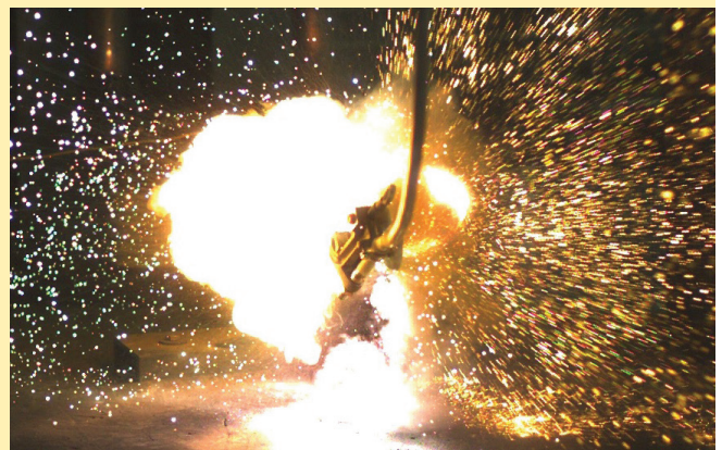
This is what it looks like when an undersized or improperly installed temporary ground set fails.
