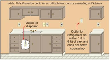
When determining distance from receptacles, distance shall be measured as the "shortest path" the cord of an appliance connected to the receptacle would follow without piercing a floor, wall, ceiling, or fixed barrier, or passing through a door, doorway, or window
