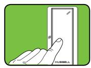
1) Press and hold switch for 6 seconds until LED flashes
