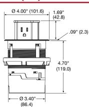
Accepts non-metallic sheathed cable and/or metal conduit (by using wire clamp or ½" KO)
