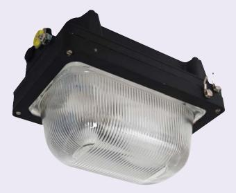
The Nexxus is a corrosion resistant bulkhead with a prismatic glass lens. It is available with a range of lamp types and is suitable for low temperature operation (-45°C). For ease of installation and maintenance the fixing points are located outside the restricted breathing enclosure.
