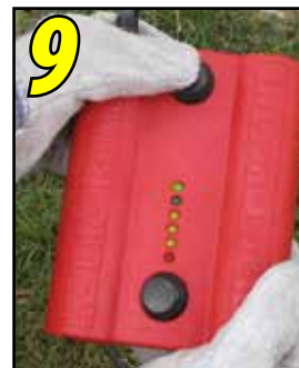
Press the "Operate" button until the exothermic reaction is initiated.
