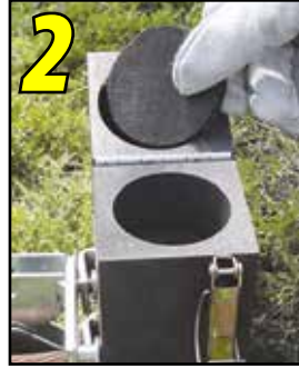
Place filter pad into lid.
