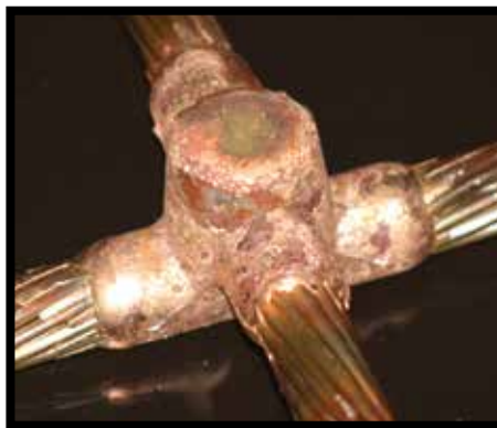
Image 1: A solid weld with only minor surface imperfections.
