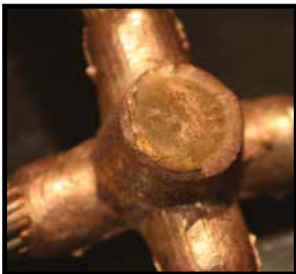
Image 2: Fill is lower than normal, but still sufficient.
