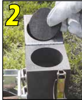
Place filter pad into lid.
