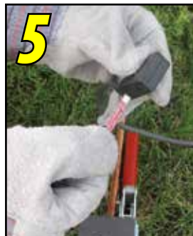
Insert the EZ Lite® Ignitor in the connector.
