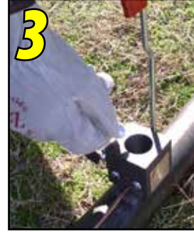
3 Place metal disc in bottom of mold.
