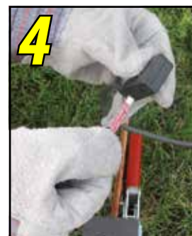
4 Insert the EZ Lite® Ignitor in the connector.
