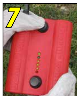
7 Press the "Operate" button until the exothermic reaction is initiated.
