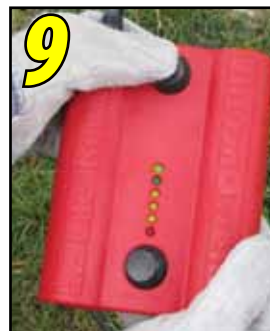
9 Press the "Operate" button until the exothermic reaction is initiated.
