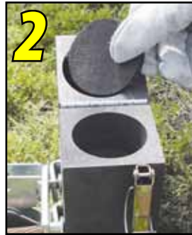
2 Place filter pad into lid.
