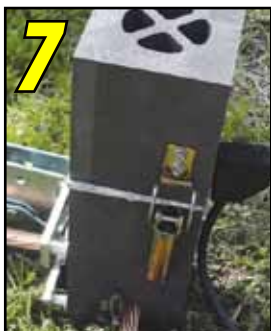
7 Close lid and secure with latch.
