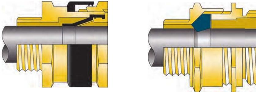
No cable damage due to Hawke 501/453 Universal diaphragm seal cable gland design.
