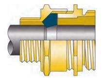
Cable damage as found with cable gland designs incorporating compression / displacements seals
