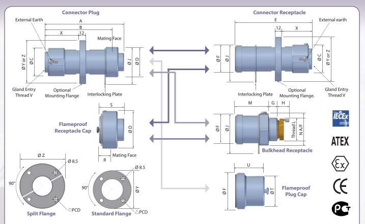
The flameproof cap must be fitted to the connector before the power is restored to the disconnected circuit. The receptacle cap and plug cap are available in acetal and provide an IP rating of IP66/67. They may only be used when the socket or plug is not re-energised following disconnection. For connector plugs and connector receptacles cable glands are required to terminate incoming cables. Hawke recommend the ICG 653/UNIV cable gland is used.
