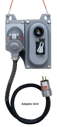
The GFCI protected ACCEPTOR® is the solution to OSHA's requirements for GFCI protection when using portable equipment in hazardous and wet locations. For use with 125V, or 125/250V③ 15 or 20 amp receptacles without GFCI protection, the **Adapter Unit** provides GFCI and circuit protection to connected apparatus by simply being plugged into an <u>existing</u> receptacle.
