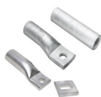
The new BURNDY® YA42A\*, YS42\* and YBA42A connectors are UL listed and CSA certified. Connectors are made of high conductivity wrought aluminum. They accommodate 900 kcmil Aluminum Class B Concentric, Compressed Compact conductors and 600 kcmil Copper Class B Concentric, Compressed Compact conductors and Class C Concentric stranding.
