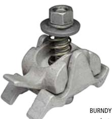
BURNDY FASTAP<sup>TM</sup> with Lineman Assist<sup>TM</sup> utilizes a spring system; that helps secure the tap conductor while installing on Primary, Secondary and Service Applications; acting as a third hand to assist in installation. The duckbill handle enables easy holding of the connector while the conductor side entry facilitates installation and helps keep inhibitor in the connector.
