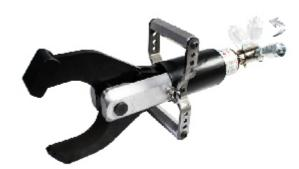
BURNDY® is pleased to introduce the all new RHCC4CUAL cutter, the first in a new series. This cutter is designed to cut Copper and Aluminum conductors up to 4.00" diameter (insulation included). The new remote head cutting tool features high strength hardened steel, scissor-action cutting blades and a unique swivel hose fitting for ease of use in confined areas.
