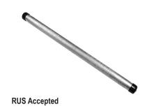
Single-sleeve aluminum UNISPLICE™ designed to splice ACSR as simply as all aluminum. Pre-filled with PENETROX™ joint compound, stripsealed and capped to limit oxide growth and to increase the life of the connection. Eliminates strand stripping, installing separate steel sleeve
