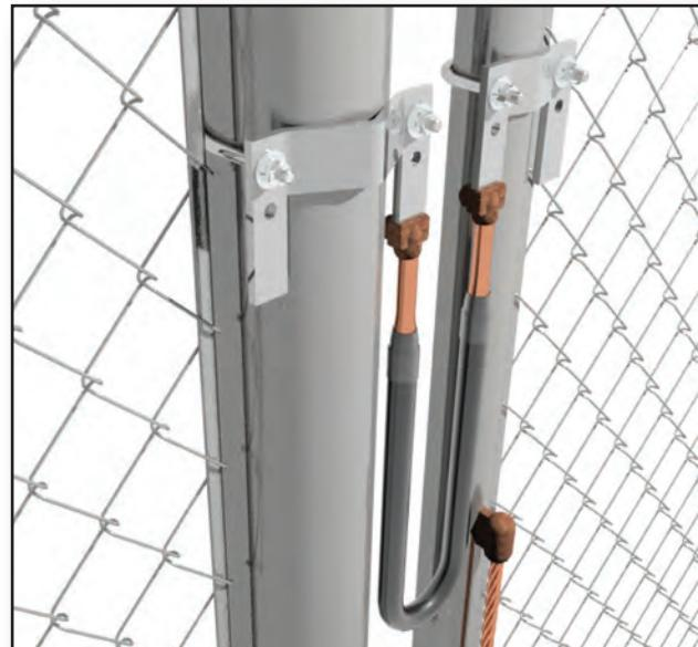
Follow the steps outlined below to specify the Fence Clamp Assembly (Exothermically Welded) you need. Replace (#) with the appropriate code from Chart A to specify the flexible jumper size. Contact factory for sizes not listed.
