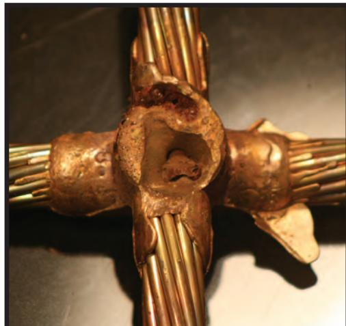
Image 5: Fill too low. Weld cavity was not filled over cable strands.
