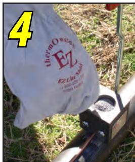
Pour weld metal into mold.
