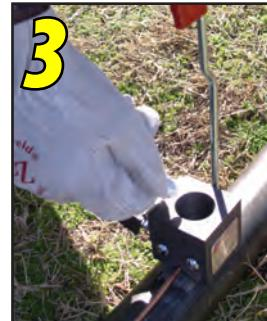
Place metal disc in bottom of mold.
