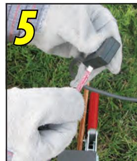
Insert the EZ Lite® Ignitor in the connector.
