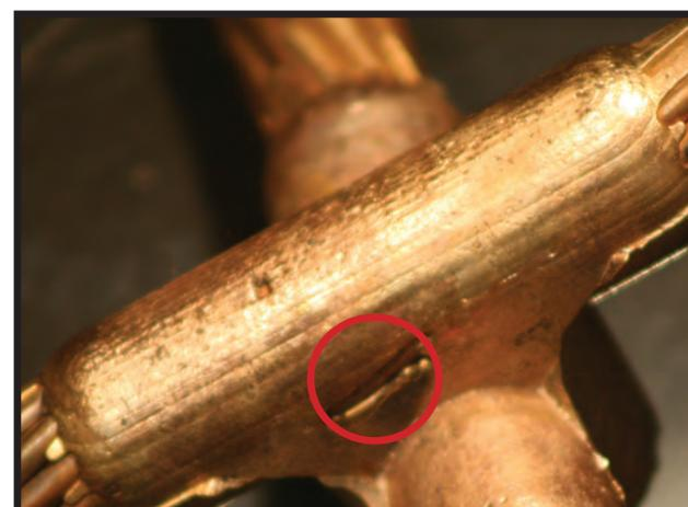
Image 7: Poor connectivity. Visible wire shown in weld.
