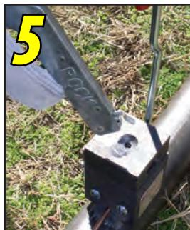
Close lid and place starting powder on top. Ignite starting powder with Flint Ignitor.
