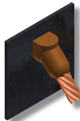
**DO NOT use Type CS-37 molds on Soil Pipe (ASTM A74-82). A test weld should be made on a section of the pipe being used to determine the possibility of detrimental metallurgical effects.**
