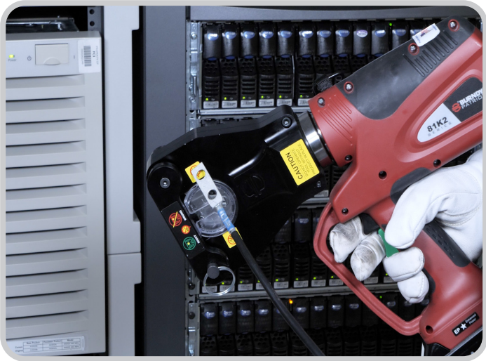
Range Taking Capability: #8 AWG to 1000 kcmil
