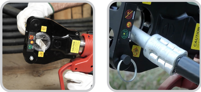
Range Taking Capability: #8 AWG to 1000 kcmil
