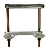
BURNDY has developed a new fence post grounding connector to accommodate 4" square fence posts. These large 4" fence post connectors are increasingly common for substation security fence applications as well as high security fences surrounding data centers, power plants, and other large industrial facilities.
