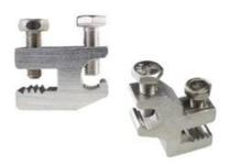
BURNDY® announces a new series of lay-in lugs - BGBS4 and BGBS5. Made of high strength aluminum alloy, these items can be used with copper or aluminum conductors. The connectors are for use with solar modules with a maximum thickness of 1/4 inches. Both are electro-tin plated and provided with stainless steel hardware.
